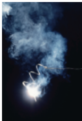
Figure 2 Magnesium reacts with oxygen to form the compound magnesium oxide. The ratio of magnesium to oxygen, by mass, in magnesium oxide is always about 3 : 2. Observing What color is magnesium oxide?
