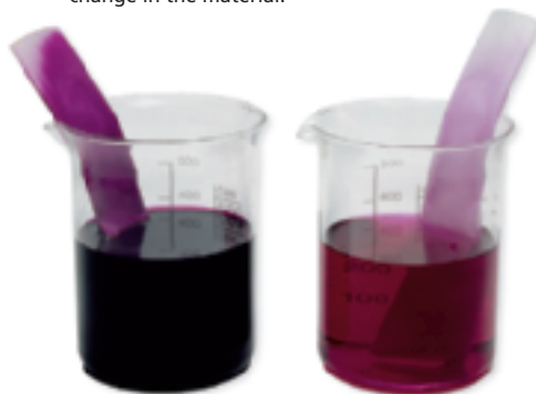
Figure 22 The dye solution in the left beaker is more concentrated than the solution in the right. Increasing the concentration of the dye increases the rate of color change in the material.
