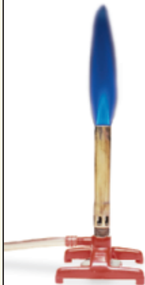
Figure 14 A Bunsen burner generates heat and light by the combustion of natural gas. Interpreting Photos What reactants or products are visible in the reaction shown above?
