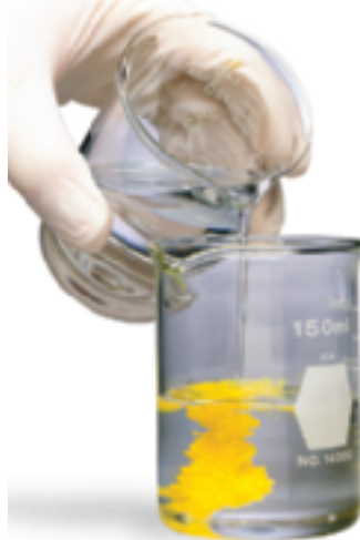
Figure 13 When potassium iodide solution is poured into a solution of lead(II) nitrate, a double-replacement reaction takes place. Lead(II) iodide forms as a yellow precipitate. Comparing and Contrasting How does a double-replacement reaction differ from a single-replacement reaction?
