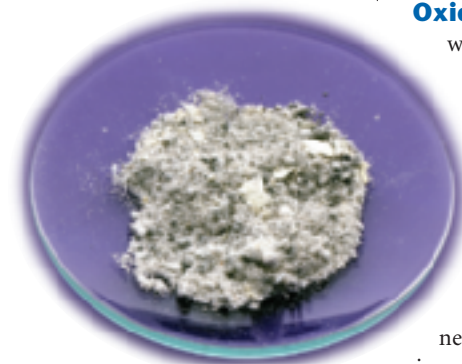
Figure 15 Calcium oxide, or lime, is produced when calcium burns in the presence of oxygen. In this reaction, the calcium is oxidized and the oxygen is reduced.
