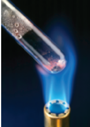
Figure 19 The orange-red powder in the bottom of the test tube is mercury(II) oxide. At about 450°C, mercury(II) oxide decomposes into oxygen gas (which escapes from the test tube) and mercury (droplets of which can be seen collecting on the sides of the test tube).
