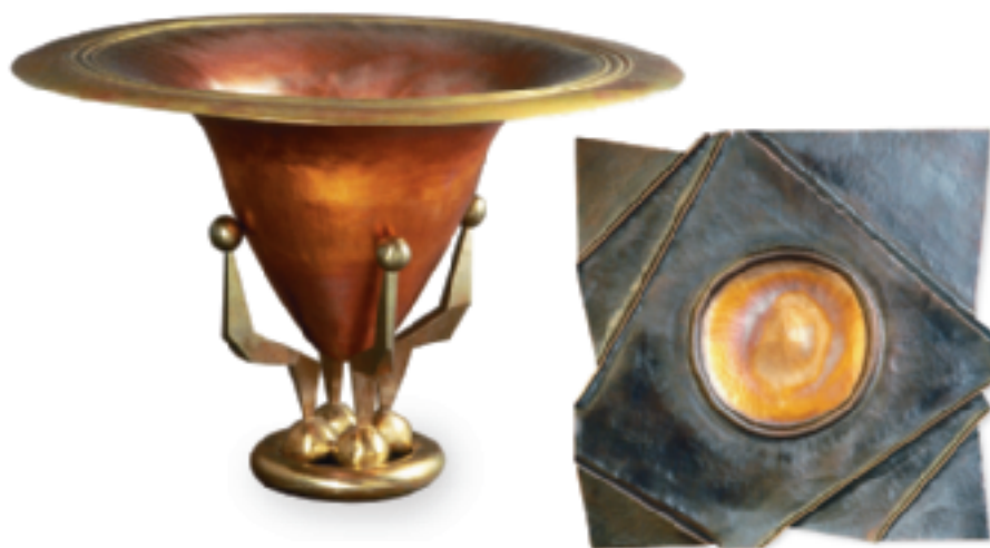
Figure 15 The brass vase on the left is coated with an oxide of copper that is red. Most of the surface of the plate on the right is coated with an oxide of copper that is black.
