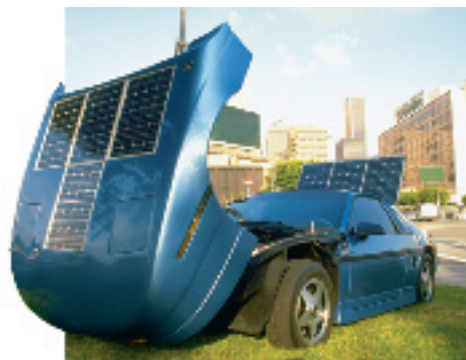
Figure 5 Panels on a solar car convert energy from the sun into the mechanical energy of its moving parts.
