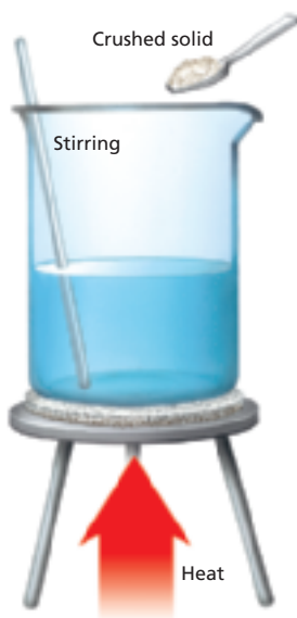
Figure 7 The rate of dissolving can be increased by reducing the particle size of the solute, by stirring, and by heating the solvent. Predicting How does changing the temperature setting on a washing machine affect how fast the detergent will dissolve?
