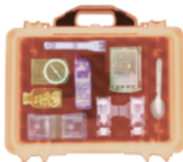
Figure 14 Airport security screeners use X-rays to search baggage for potentially dangerous objects. Inferring Why are there dark areas in this X-ray image?
